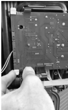
Step 4 Snap the PCB back into place
