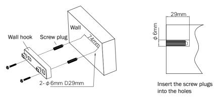
3 Attach the product on the hook through the large mounting hole and securely mount it by moving right to the position of the small mounting hole.
