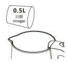
2. 倒入0.5L食用白醋,浸泡1小時以上。 Fill the kettle with 0.5L white vinegar. Leave the solution in the kettle for at least 1 hour.
