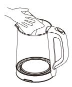
3. 倒掉壺內白醋,用濕布擦去殘留的沉澱物。 Discard the vinegar and rub the stains with a damp cloth.
