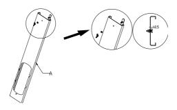
Slide the extension panel between the main panel and the screw's 2.5mm gap and adjust the length needed to cover the window opening.
