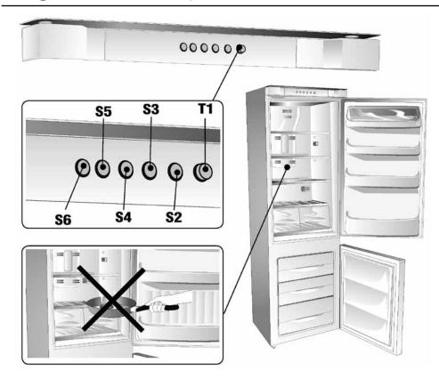
Temperature programming and control: different temperatures can be selected, as indicated by the 3 green leds (S2-S3-S4). To change settings, press button (T1); on each click the illuminated led turns off and the next one flashes for 4 seconds according to the sequence S2-S3-S4 - S5. The new setting is saved at the end of the flashing phase. Activation of SUPER mode (S5) is by means of button (T1) after which the yellow led (S5) is permanently lit.
