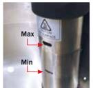
2. Fill the container with water. The water level should be between the Min and Max levels indicated on the front of the circulator. According to the Archimedes's principle, the water level will rise when food is added to the container, so don't fill it up too high.
