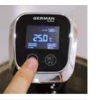
3. **Press the control panel**. Press the Power (b) button for more than five seconds. The first line display will then show the set temperature of the water, the second line the current temperature. The third line will show the set time and work time.
