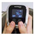
3.2 Celsius or Fahrenheit: Select either Celsius or Fahrenheit as the unit of measurement. Press Power 1 button and Set  $\textcircled{\text{RET}}$  button at the same time for two seconds to select.
