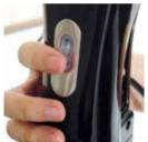
4. Set the temperature and time. Scroll up the scroll wheel to increase the set temperature and time, and scroll down to decrease. The maximum temperature setting is  $95^{\circ}\text{C}$  or  $203^{\circ}\text{F}$  and the time setting ranges from 00:00 to 59:59.
